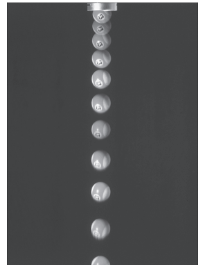
FIGURE 2.11 Strobe photo of a falling ball. Successive images are farther apart, showing that the ball is accelerating.
