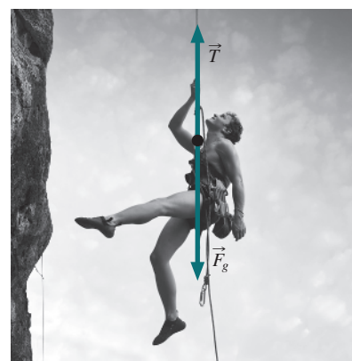
FIGURE 4.6 The climbing rope exerts an upward tension force \vec{T} that balances the force of gravity.
